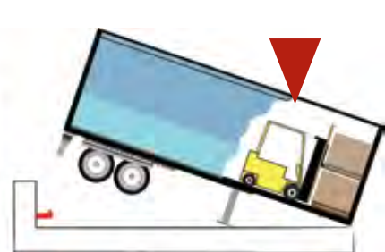
3. Trailer tips forward Once center of gravity is in front of landing legs, nose-dive is imminent.
