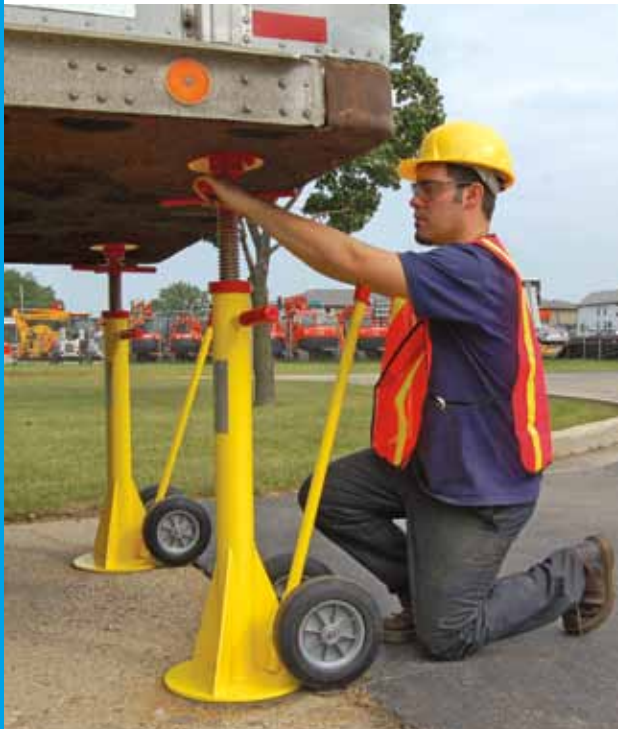
Install a pair of jacks at front of trailer against the smooth underfloor and always in front of the kingpin.
