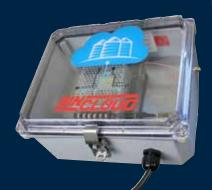
The BinCloud Gateway is also designed to accommodate sensor devices under development for the future. LoRabased ultrasonic and radar level sensors and camera-based level scanning solutions will utilize the BinCloud Gateway.
