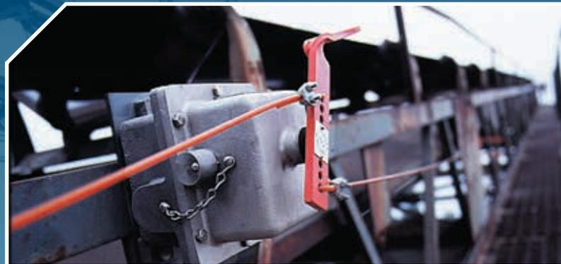
As shown in the chart and picture of the actuating arm, the actuation force can be varied by attaching the cable at any one of the three positions.
