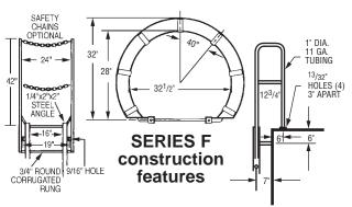
SHIPPING NOTE: All 15 thru 25 rung Series F models with cages ship in 2 sections. All 26 thru 30 rung models ship in 3 sections.
