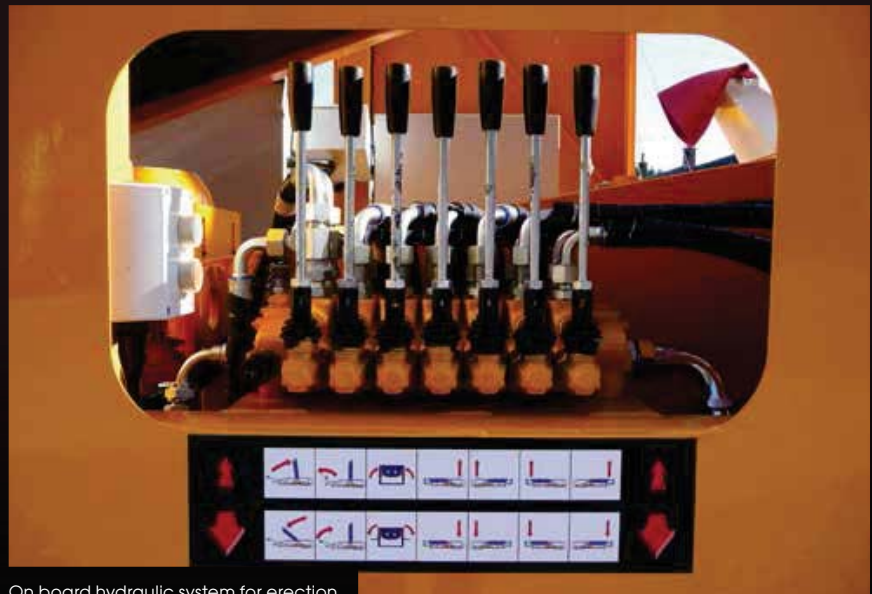
On board hydraulic system for erection
