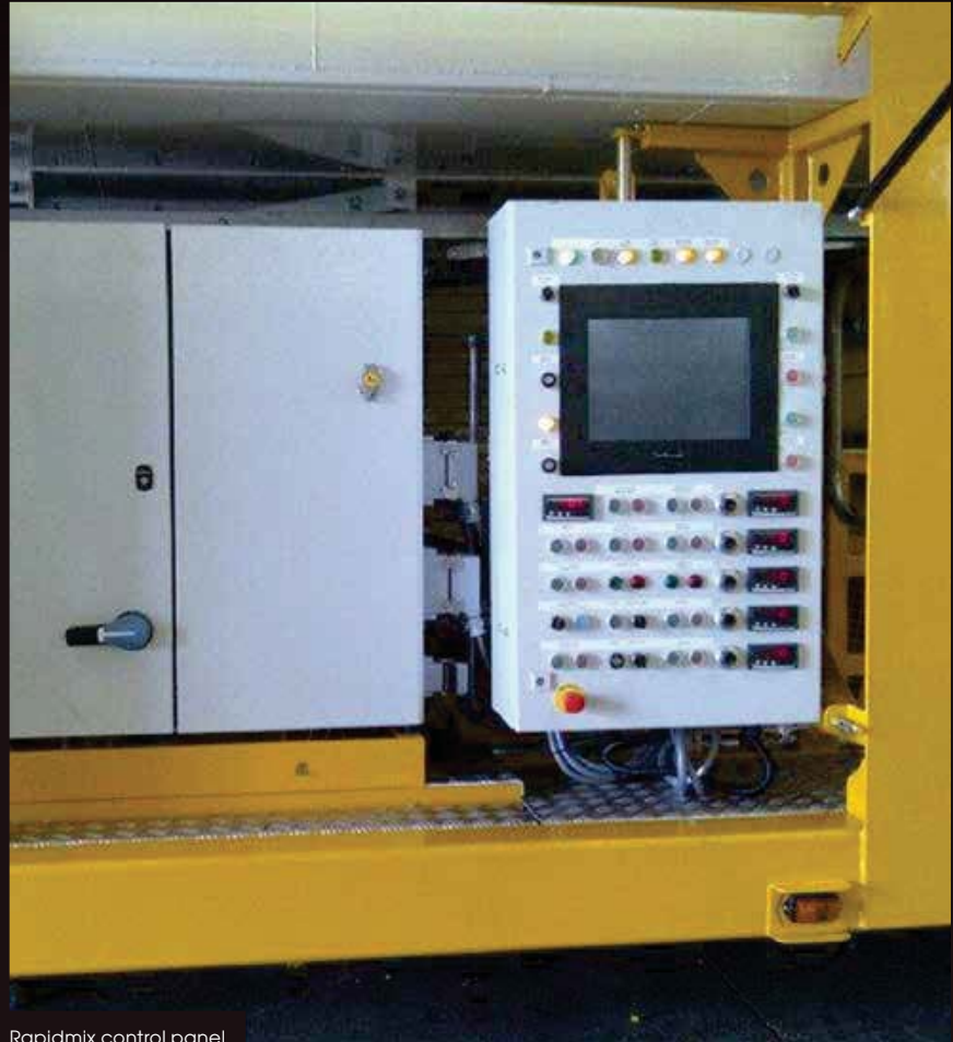
Rapidmix control panel
