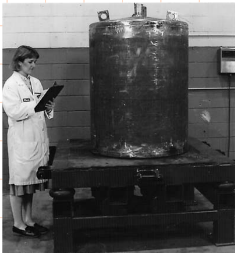
Vibrating table used to test density and material weight for each load. Table also tested for weldment cracks and fatigues during a normal 24 hour test cycle.
