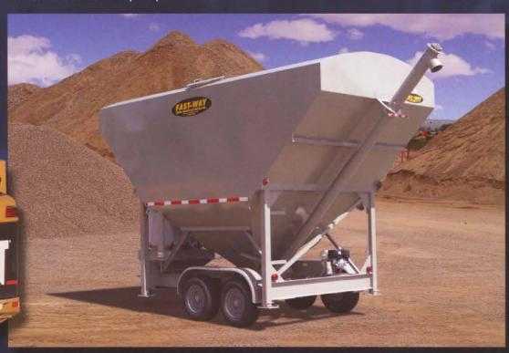
For the process of filling a fleet of site mix-trucks, the SI-LOW 206 or SI-LOW 210 is ready to perform as a portable fill station. The SI-LOW 206 stores 200 barrels of cement and discharges the cement with a 6" auger. The SI-LOW 210 also stores 200 barrels of cement, but has the advantage of increasing cement-discharge with a 10" auger.
