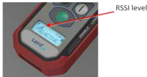
Figure 4: RF Signal Level Monitoring
