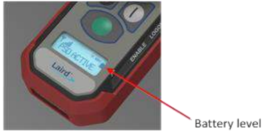
Figure 5: Battery Level Monitoring
