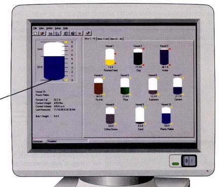
Provides a graphical representation of 10 vessels per tab, plus detailed inventory information on a single vessel.
